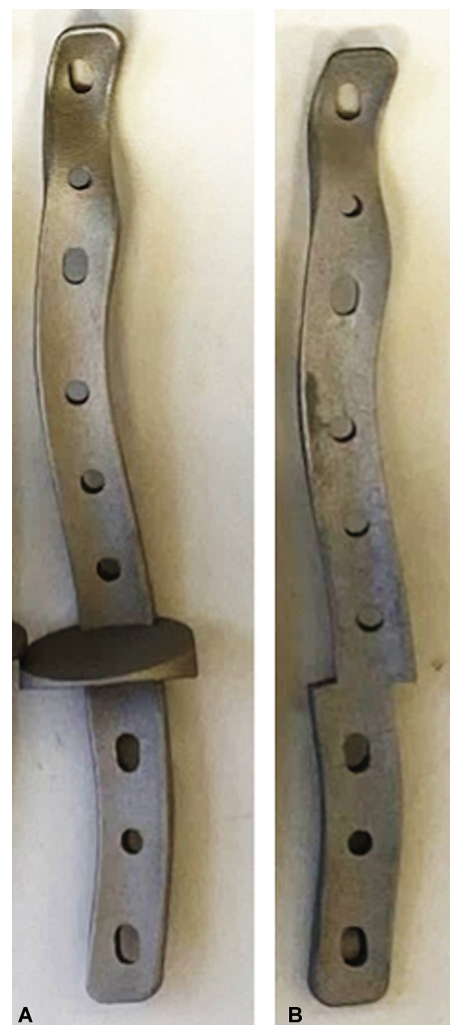
Fig. 3 Three-dimensional (3D) printed sample-specific implants showing an (A) opening wedge construct and (B) a rotational construct. The implants shown are 75% the length of the humerus straight osteotomy plates.
