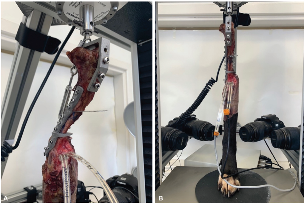
Fig. 7 (A,B) Photographs of the testing setup for the 75% oblique 10-degree medial opening wedge construct. The plate is applied to the medial aspect of the bone with eight 3.5-mm bicortical screws and one 3.5-mm monocortical screw. At the location of the 50% osteotomy, an oscillating saw blade is left in place to fill the space left by the saw kerf and prevent limb shortening. The ultra-thin sensors can be seen along with their connections to the microcontroller board. The custom-designed mount is secured to the proximal humerus with three 4.5-mm bicortical screws and fits into a custom-designed socket to simulate the shoulder joint. The paw is positioned on sandpaper under which are four screws that aided repeatable paw positioning.
