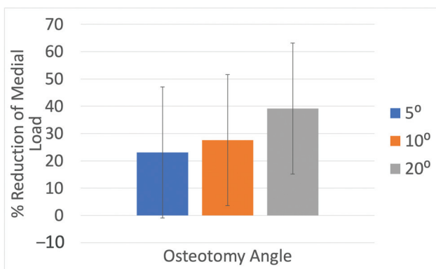
Fig. 12 Percentage reduction of load through the medial compartment depending on angle of change induced by the construct. This graph compares all 5-degree constructs with all 10-degree constructs and all 20-degree constructs, including all osteotomy directions, levels, and types.
