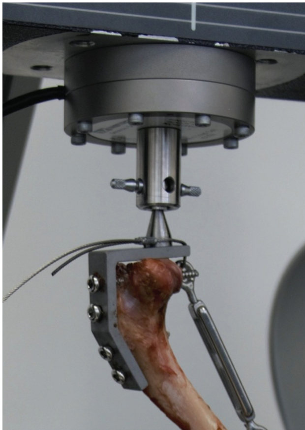
Fig. 5 Custom-designed mount with custom-designed socket for universal testing system. The mount was secured to the proximal humerus using three to four 4.5-mm cortical screws. The mount has a conical point that articulated with the custom-designed socket that was attached to the loading device. The turnbuckle apparatus mimicking the pull of the triceps is also appreciable; this was attached to the mount using a loop of stainless steel wire (all pictured).
